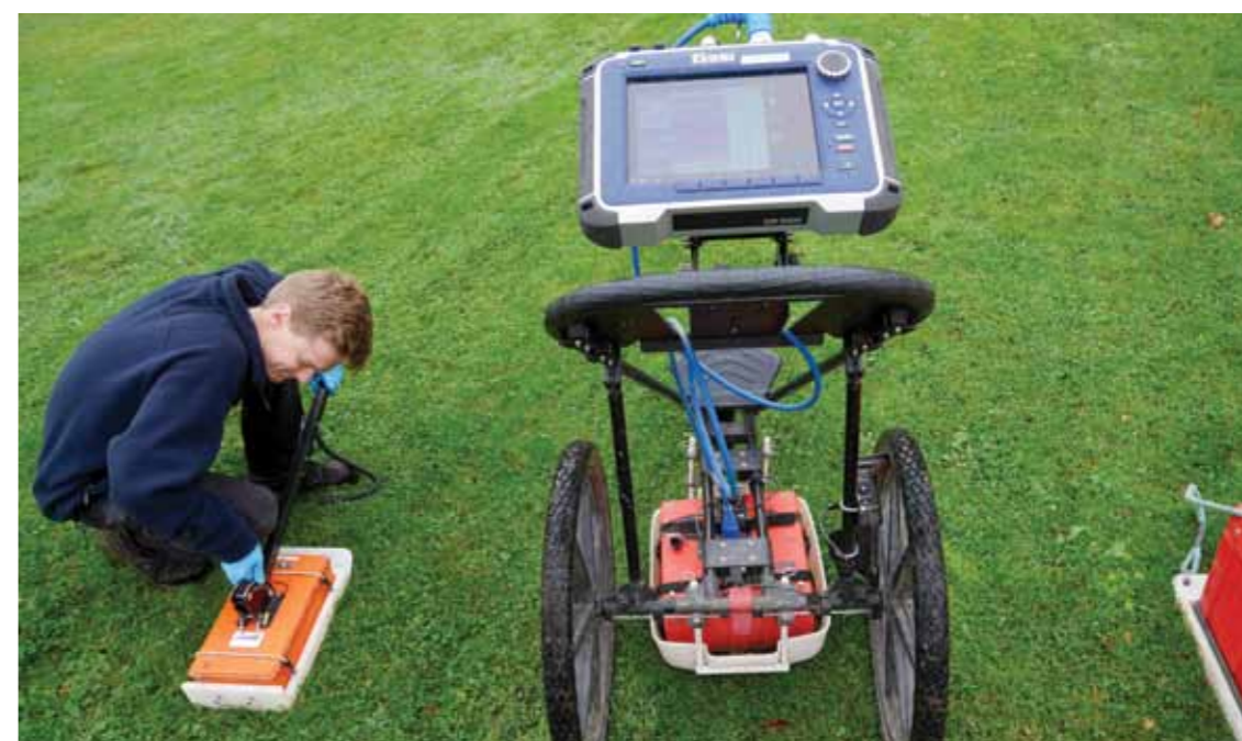
PICTURE: COURTESY PAUL JAMESON: LIAM WILLIAMS OF RSK STATS SETS UP A MOBILE GPR DEVICE
